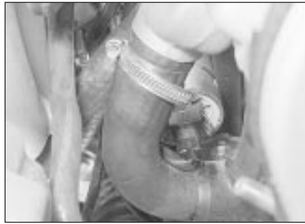
13.27b . . . and the large coolant hose
