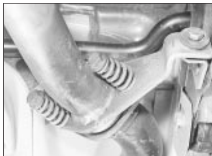
14.5 Manifold-to-exhaust system joint and bracket
