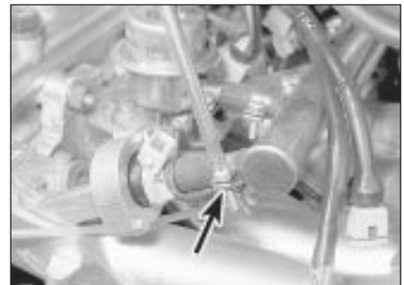
12.6 Slackening a fuel rail hose clamp
