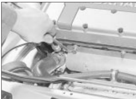
14.3 Removing an exhaust manifold heat shield bolt
